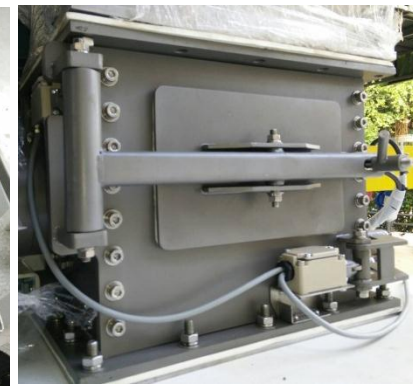
Safety switch for door opening protection
