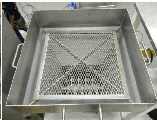
Safety screen for low loading hopper
