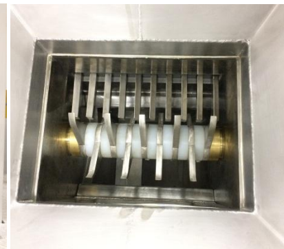
Removable breaking finger, Option for cutting feature
