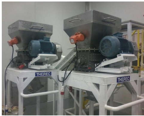
Complete unit with moveable metal bas and loading hopper
