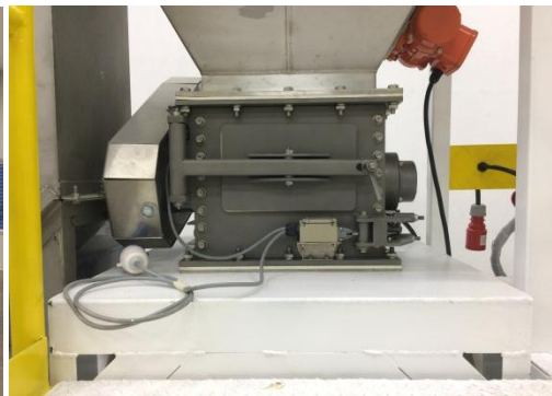
Vibrating motor for low loading hopper
