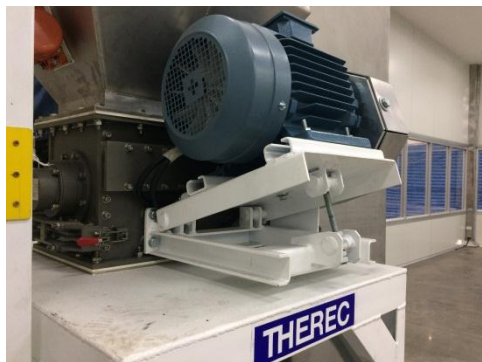
Adjustable motor base for belt tensioning
