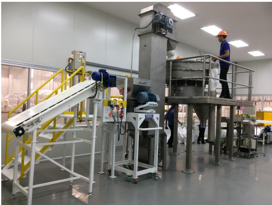
Complete station with Control panel with frequency inverter, Low loading hopper and top cover, Metal base with wheel and lockable stand, Operation platform, Bag laying table, Hand rail and Stair
