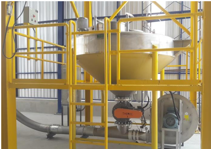
Special Design / with 2 Monorail Hoist and Extra large buffer hopper of 4,000 liter
