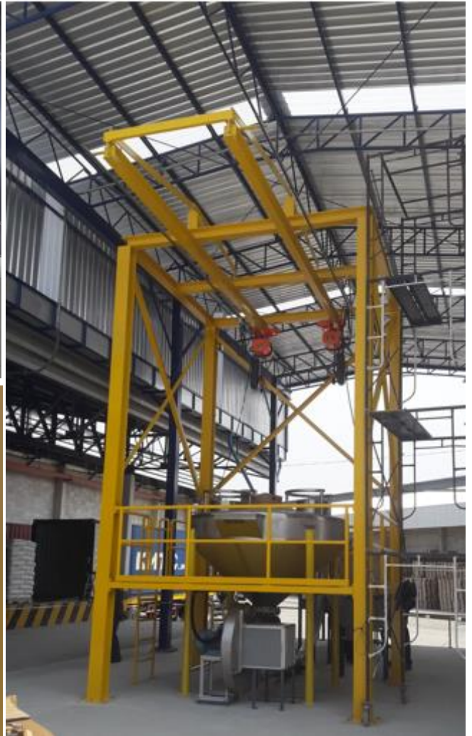
Special Design / with 2 Monorail Hoist and Extra large buffer hopper of 4,000 liter
