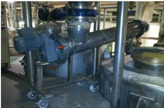
Easy clean screw conveyor AB Food (Thailand) Ltd. / Ovaltin Sugar + Malt + Milk powder
