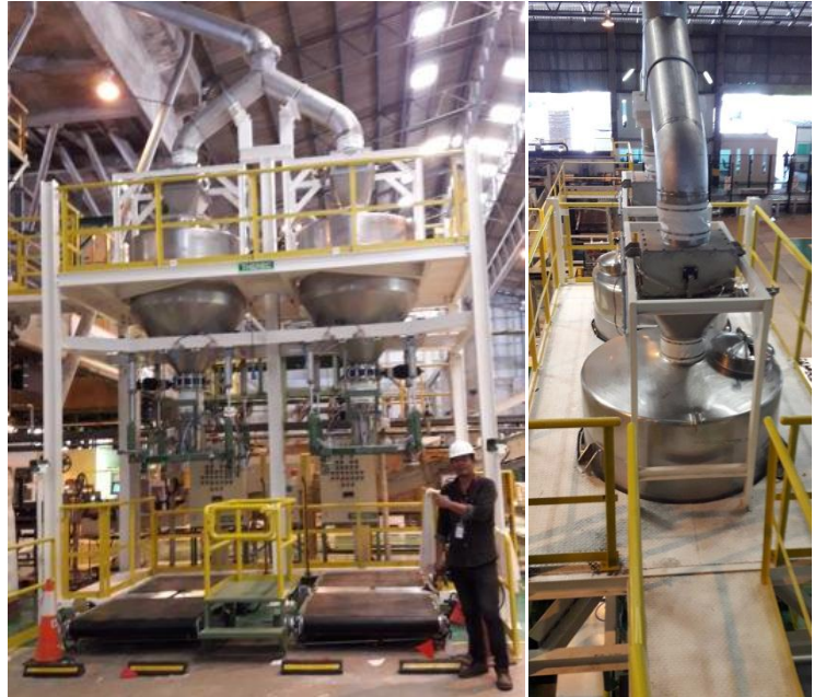
Big Bag Filling & Weighting Station / High Speed / Platform Scale
