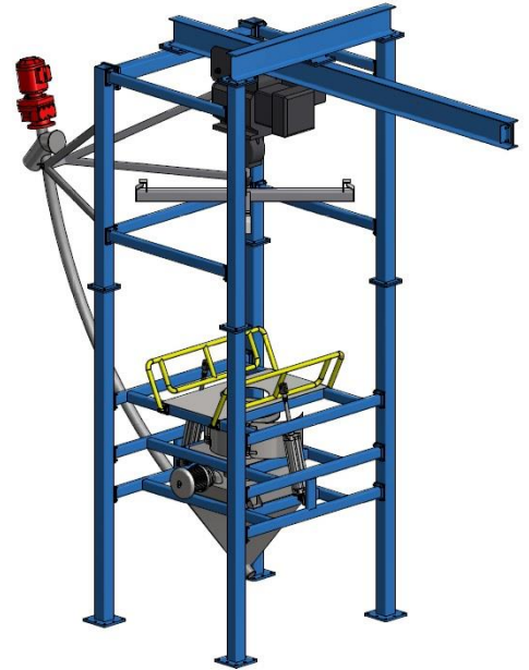
Special Design / Monorail Hoist Big Bag Unloading Station
