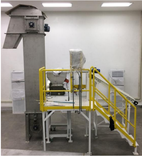
Complete station with Control panel with frequency inverter, Low loading hopper and top cover, Metal base with wheel and lockable stand, Operation platform, Bag laying table, Hand rail and Stair
