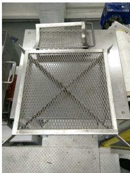
Easy Removable, Light weight design in all screens items for Cleaning and Unblocking purpose
