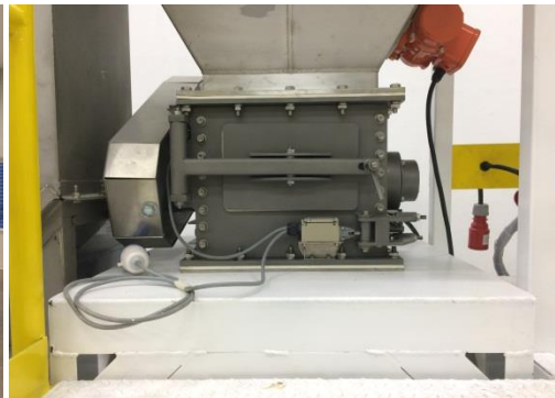
Vibrating motor for low loading hopper
