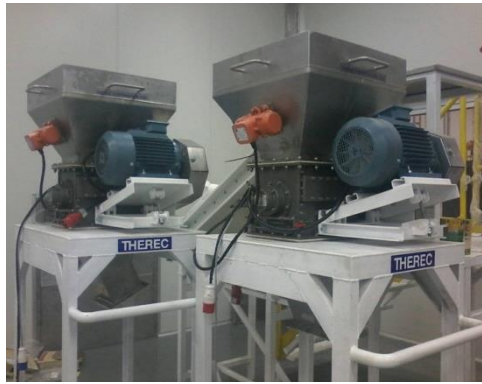
Complete unit with moveable metal bas and loading hopper
