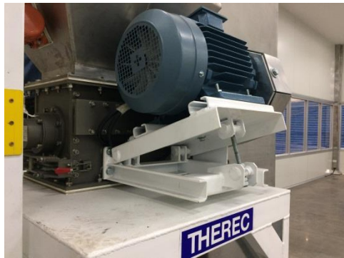
Adjustable motor base for belt tensioning
