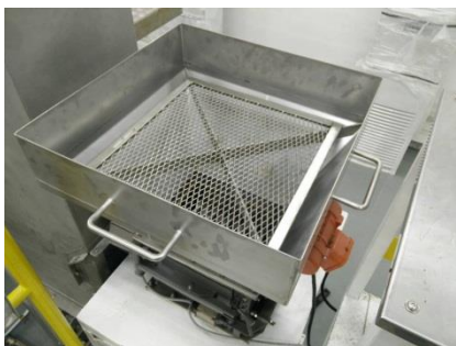
Easy Removable, Light weight design in all screens items for Cleaning and Unblocking purpose
