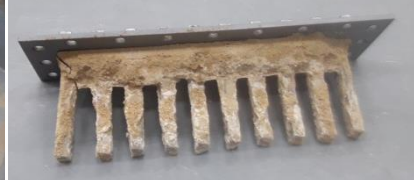
Easy Removable, Several type designed Edge cutting finger, increasing the breaking efficiency www.thereccorp.com
