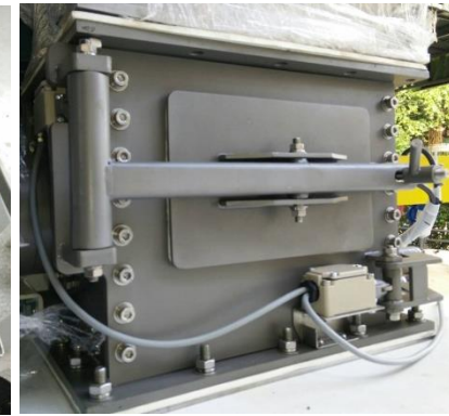
Safety switch for door opening protection
