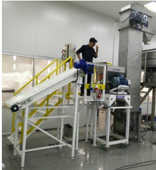
Complete station with Control panel with frequency inverter, Low loading hopper and top cover, Metal base with wheel and lockable stand, Operation platform, Bag laying table, Hand rail and Stair
