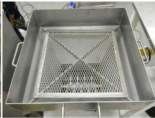
Safety screen for low loading hopper
